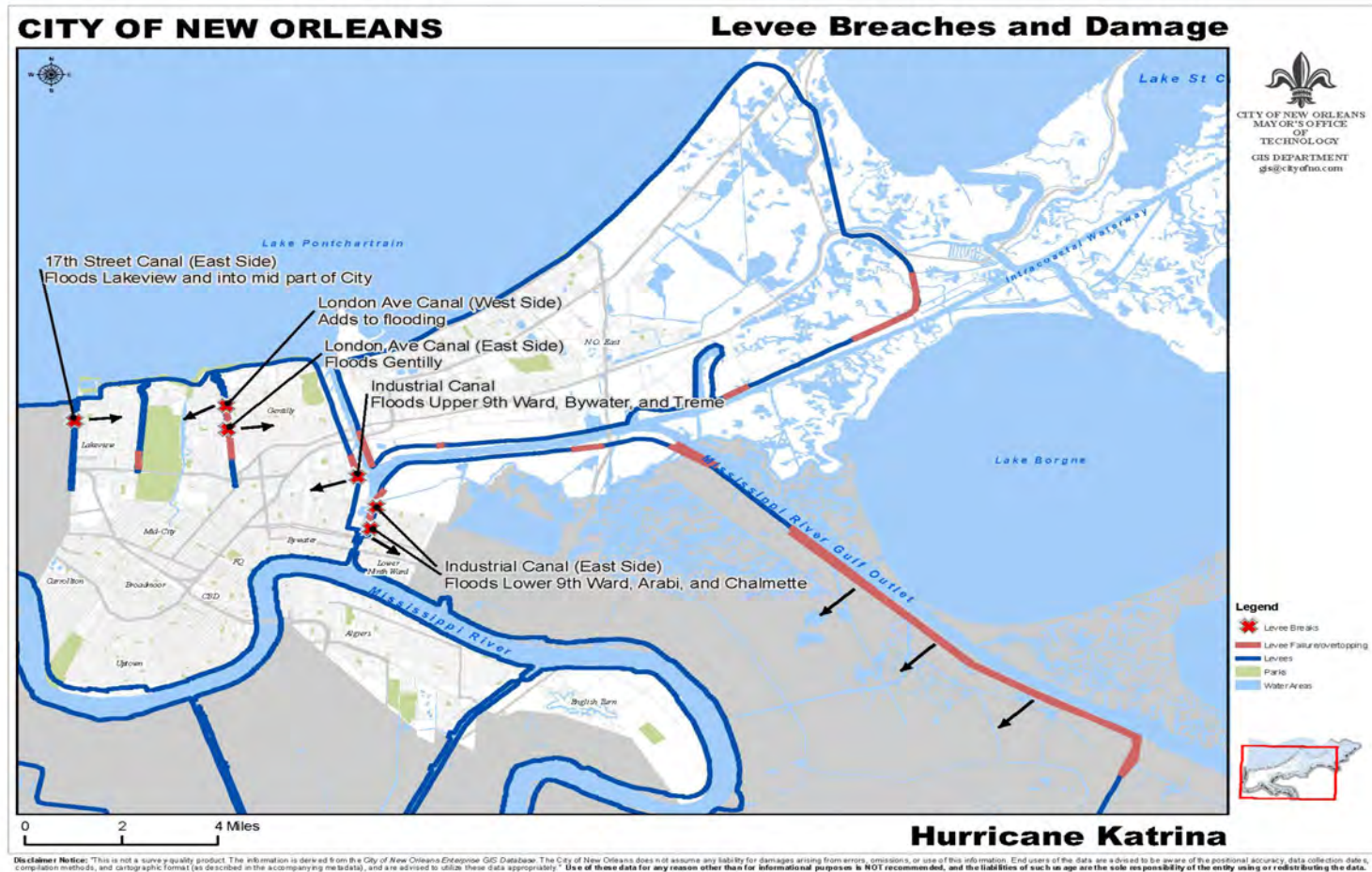
Figure 19: New Orleans Hurricane Risk Reduction System, with Locations of Levee Failures caused by Hurricane Katrina in 2005
